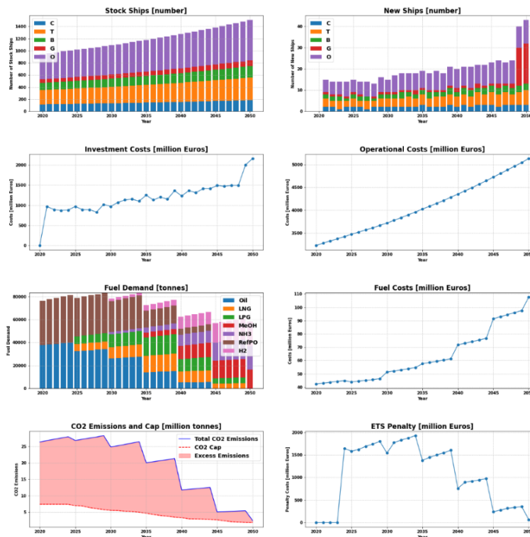
Figure 1. Results of the application to the Greek fleet, including: the fleet composition; investment and operational costs; fuel demand; the CO2 emissions compared to the ETS threshold, and the associated penalty.
