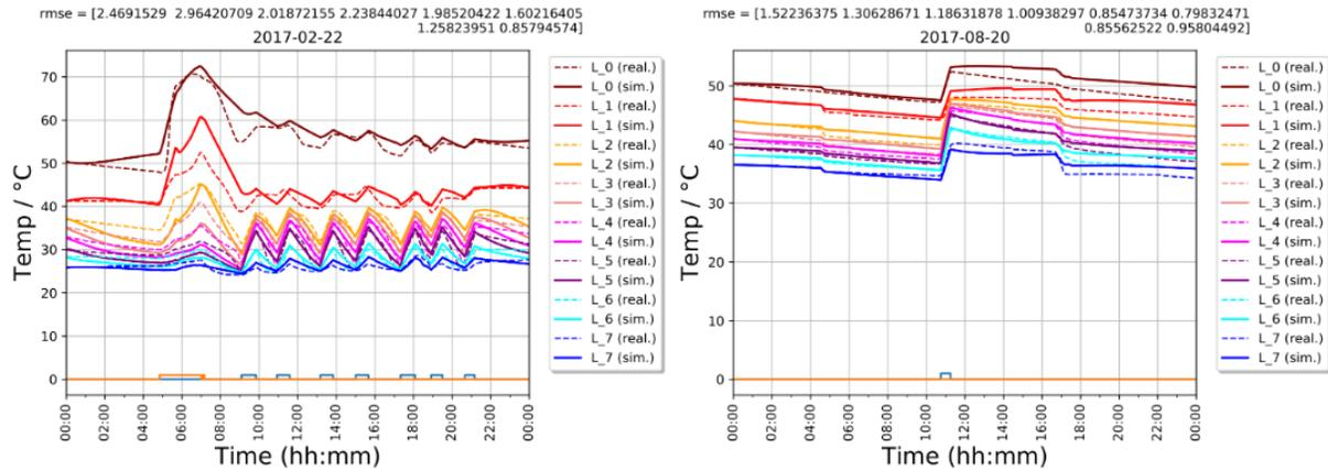
Figure 1. Simulation with one step ahead prediction. Depicted are the real vs. predicted values with the LSTM-ANN model. The starting conditions are the temperatures at the beginning of each day. On the left, a winter day simulation is showcased, on the right a summer day.
