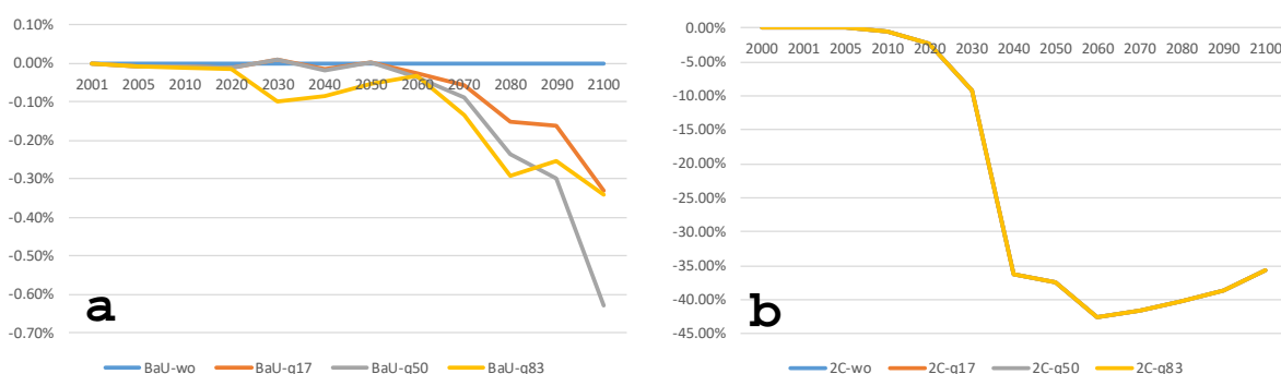
Fig. 4 Total primary energy supply in the world relative to the BaU-wo case. (a) BaU scenario, (b) 2°C scenario.
